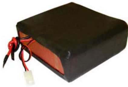
Figure 8 58.8[V] Lithium Ion battery pack
